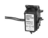
The device is designed to protect circuits from harmful voltage drops. It can also be used for remote control purposes. The trip operates when the voltage drops to less than 70% of nominal coil rating, and the breaker cannot be reset until the voltage recovers 85% of its normal rating. See page 06/70.
